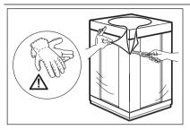
1. Remove the external film. If necessary, use a cutter.
